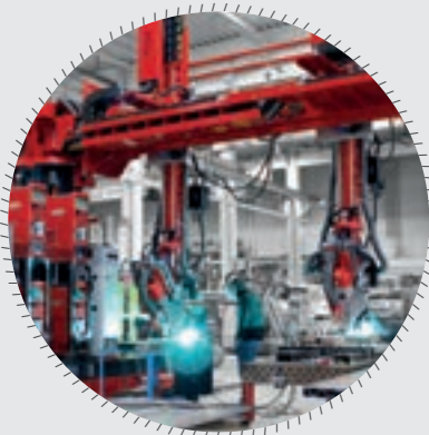
LINEAR WELDING SYSTEM 10 AXES
