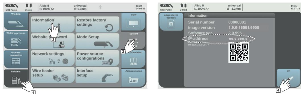
**[1]** Presettings/System/Information ==> note down IP address of power source
