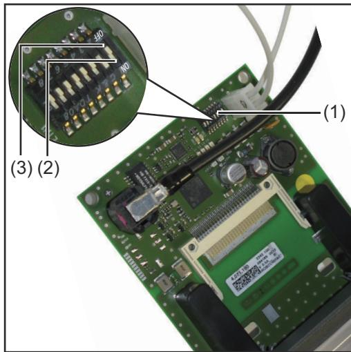
The dip switch (1) on the robot interface RI FB Inside/i is used to configure
