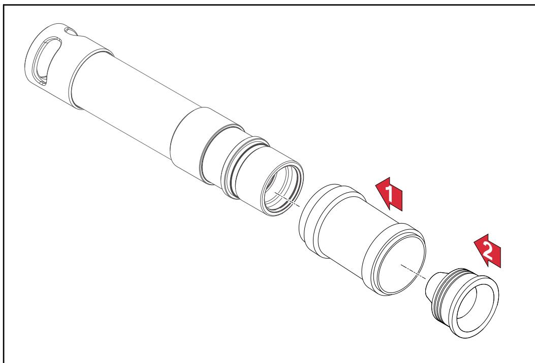
Fitting the shaft seal and the slide coupler to the Exentometer is only required for volumetric flow measurements on non-Fronius products.
