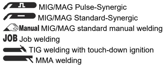
**IMPORTANT!** If the VR 7000 wirefeeder is connected to a TS 4000/5000 power source, MIG/MAG pulse synergic welding is not available.
