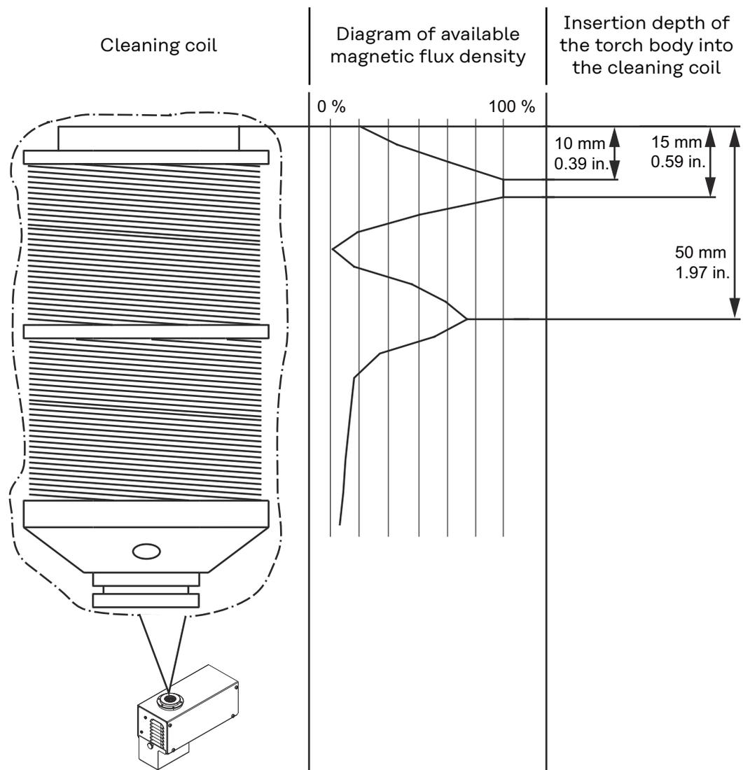
**Representation of the magnetic flux density within the cleaning coil for twin applications**
