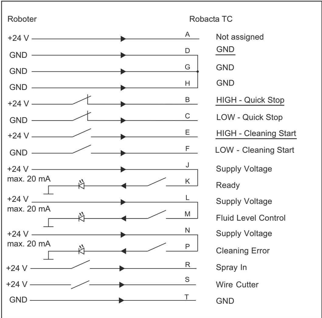
Standard I/O (X1) connecting plug configuration
