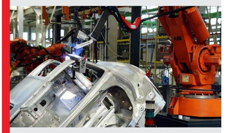
"By using CMT Advanced we can avoid the problems we had previously been having with porosity on joints involving castings."
